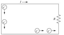
The power dissipated in a resistor is given by  $P=I^2 R \label{eq:power}$
