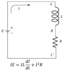
The first term is the rate of increase of the magnetic energy. The second term is the power dissipated as heat.
