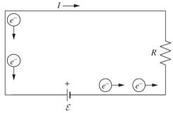
The battery is a source to continuously provide a non-electrostatic field to push charges moving through the circuit. The source is called an electromotive force (EMF) on the circuit. [c.f.4-3]
